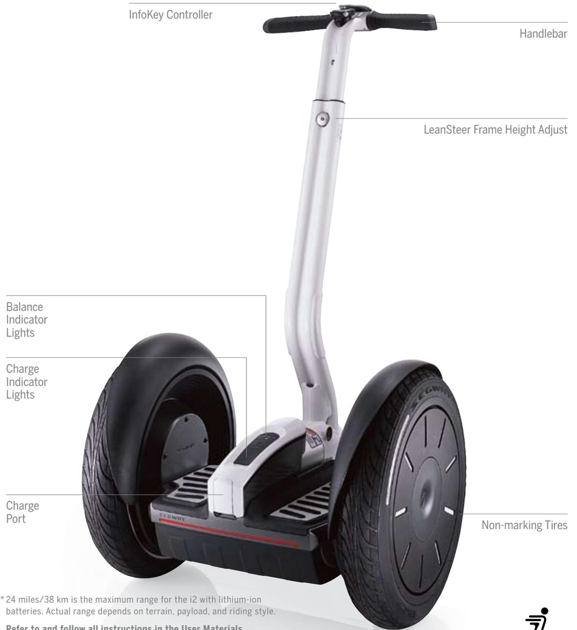
\* 24 miles/38 km is the maximum range for the i2 with lithium-ion batteries. Actual range depends on terrain, payload, and riding style.
